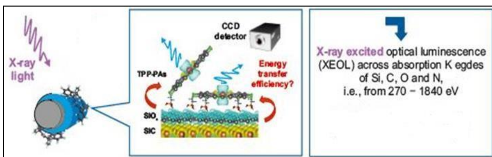
Figure 17: XEOL technique to determine the conformation of porphyrins on metallic supports
