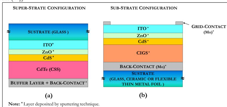
**Figure 1** Structure of (a) a CdTe- and (b) a CIGS-based solar cell.
