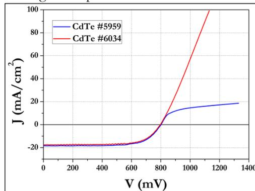
**Figure 3** Comparison between sample CdTe #5959 (external contact is made without platinum) and sample CdTe #6034 (external contact is made with platinum). J-V characteristics were measured under the Standard Test Condition (STC) – namely, incident power density of 1000  $\text{W}/\text{m}^2$ , a temperature of 298.15 K, under AM 1.5 filtered solar light spectrum.
