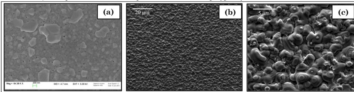
**Figure 2** Morphology SEM images of: (a)  $3 \mu\text{m}$ -thick CdTe film deposited using CSS, (b)  $3 \mu\text{m}$ -thick CSS-deposited CdTe +  $200 \text{ nm}$ -thick sputtered CdTe, (c) the film (b) after a heat treatment at 670 K under a controlled chlorine atmosphere.
