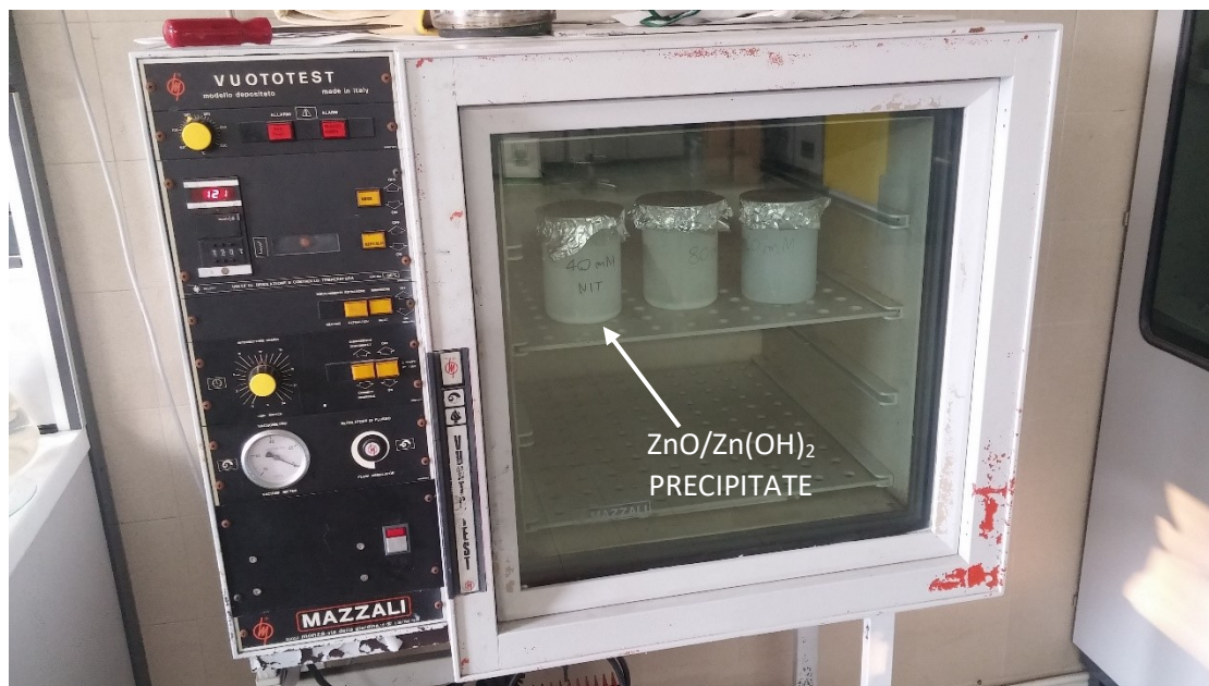
Fig. 42: Growth solutions into the vacuum oven. A white layer is visible at the bottom of the beakers, which is caused by deposition of Zn(OH)_2 formed by the alkaline environment originated from HMTA decomposition, and nano/microstructures grown through homogeneous nucleation. These are usually bigger in size with respect to the NRs that grow on the substrate surface, so precipitation occurs despite convective motions. These are, however, responsible for the cloudy appearance of the solution, since smaller nanostructures are transported within the solution.
