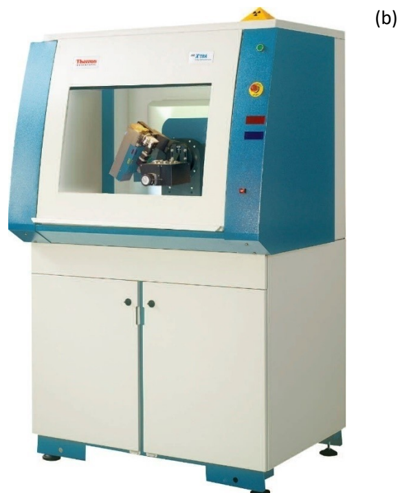
Fig. 38: (a) Bragg-Brentano \theta - \theta geometry in a XRD system. (b) Thermo ARL X'tra diffractometer.
