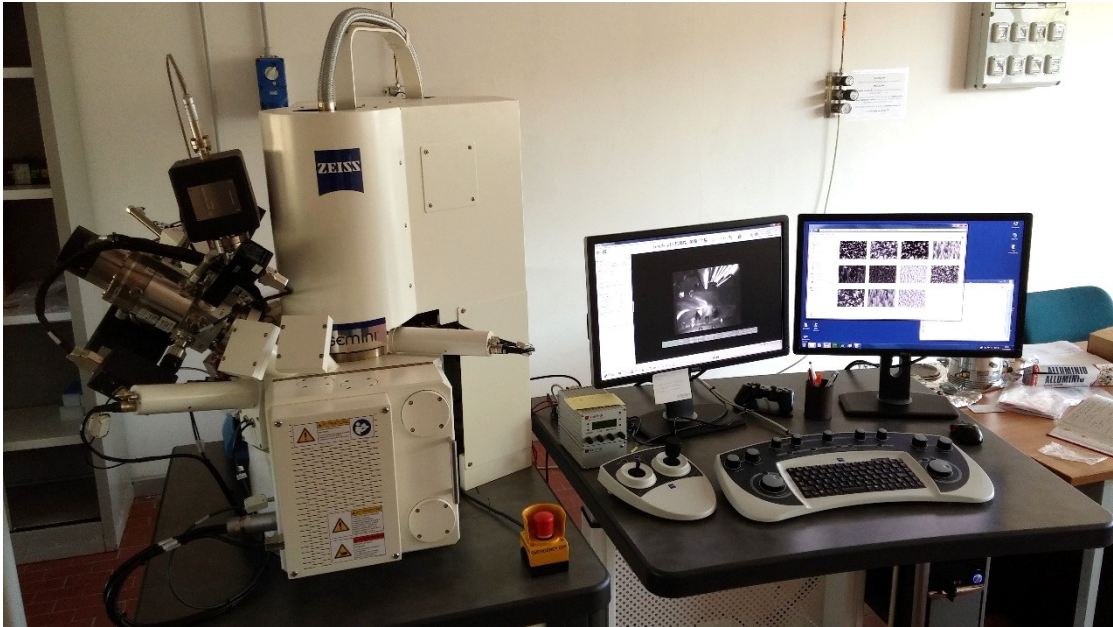
Fig. 32: The dual beam Zeiss Auriga Compact system equipped with a GEMINI Field-Effect column used in this study.
