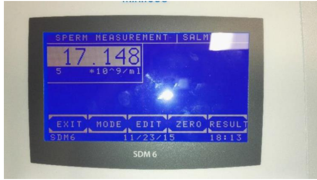
Figure 2.7: picture of the photometer SDM6 (by Minitüb GmbH and Cryogenetics®) showing the data output. In the example the measurement of the milt concentration is 17.148 \times 10^9 /ml.
