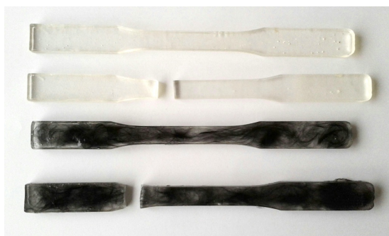
Figure 35: Broken and intact samples of epoxy thermoset with (bottom) and without (top) CF-nanohybrids.
