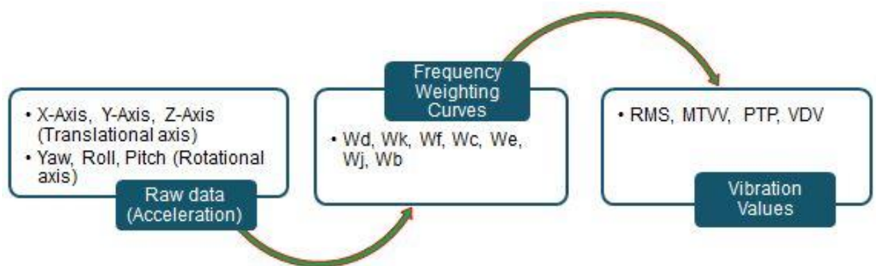
Figure 34: Flow chart for vibration data processing.
