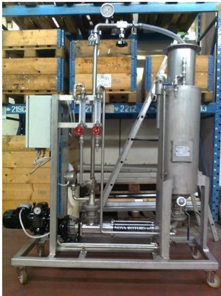
Figure 19: The degumming wastewater processing prototype
