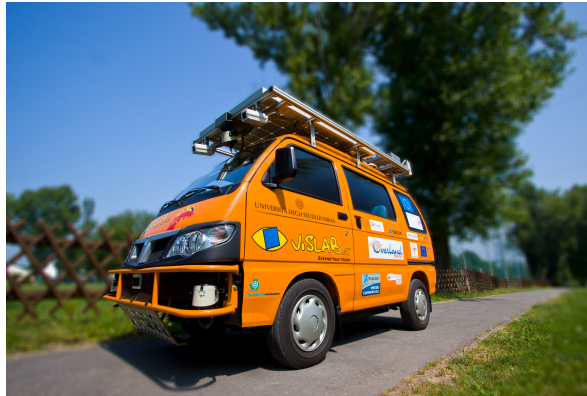
Figure 2.13: Autonomous Piaggio Porter. It mounts several stereo vision systems, with different baselines, that look in different directions. It also has four laser scanner that cover the area all around the vehicle
