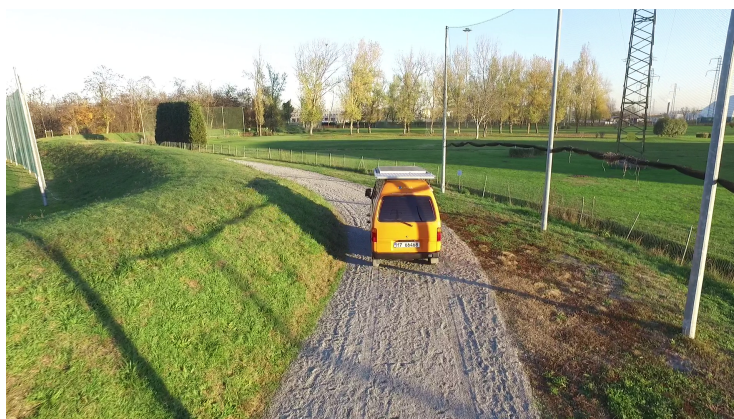
Figure 3.28: Example of result of Target Tracking Algorithm. In this case the drone is following a vehicle on an untarmacked road.
