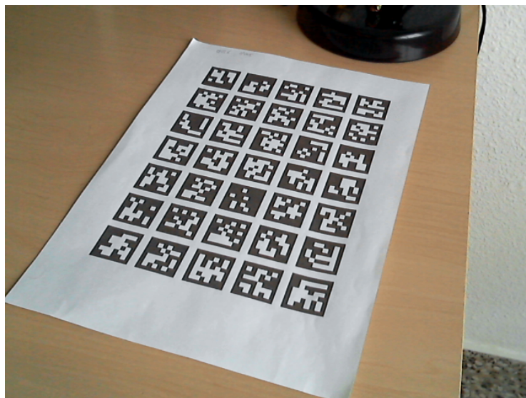
Figure 3.30: Example of ArUco marker board.
