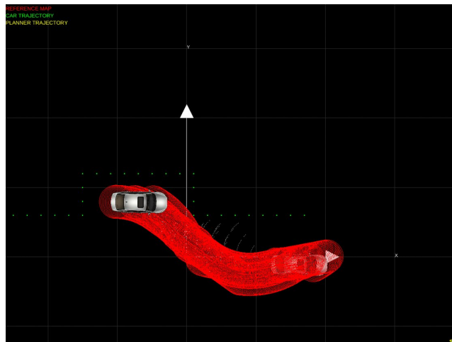
Figure 2.21: Simulation of an parallel park. The space occupied during the maneuver is shown.
