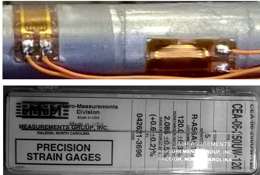
Figure 2.9. Strain gauges glued to the beam and their datasheet.
