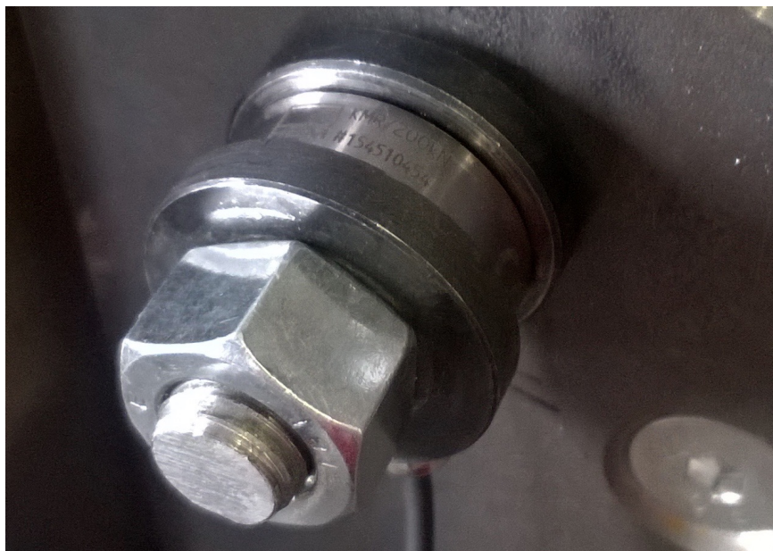
Figure 2.14. Load cell mounted on the beam.
