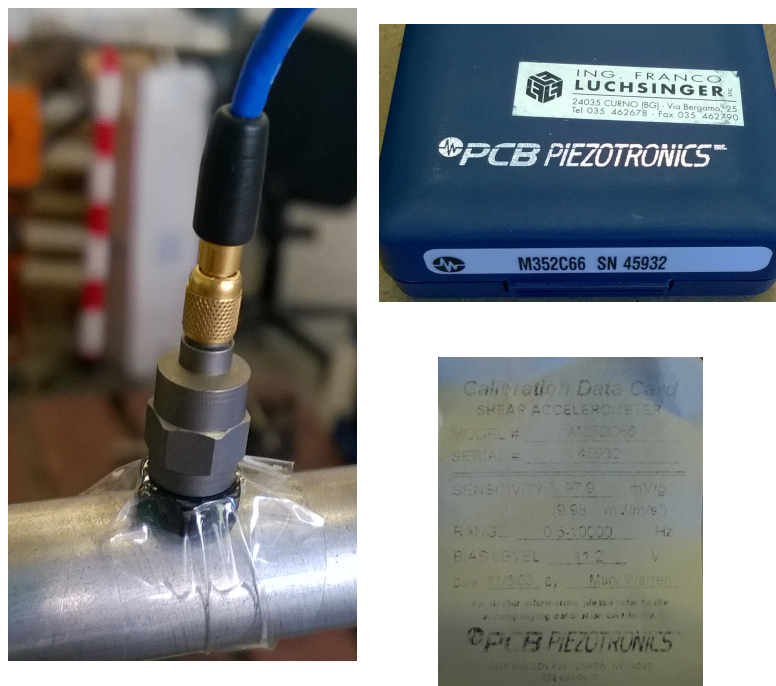
Figure 2.19. Accelerometer used for dynamic response acquisition.
