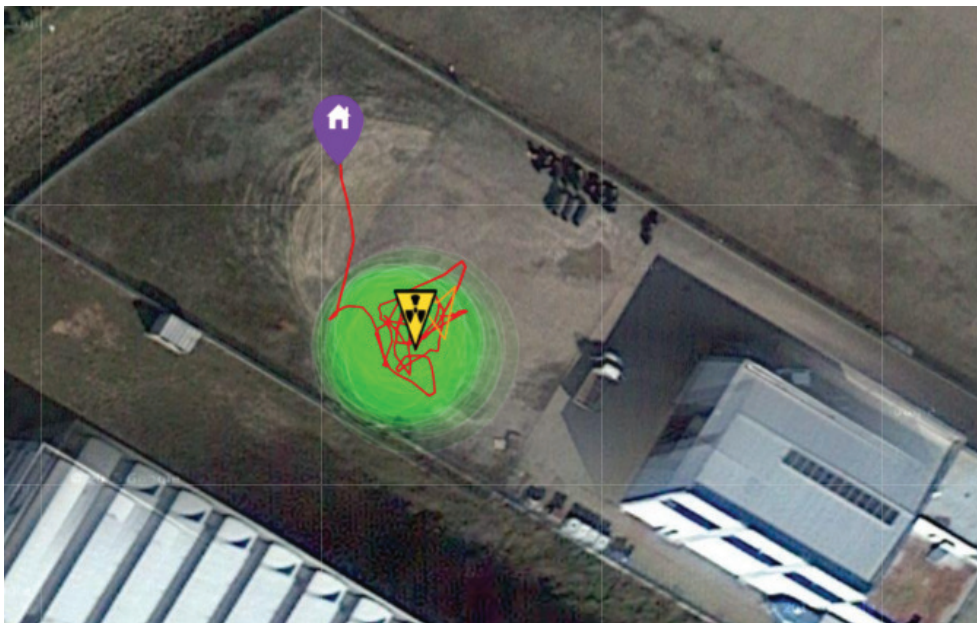
Figure 4.18: Detection of Iridium 192 in real environment (operator has direct sight of the nuclear source): flight path, regions where a radiation was measured by the CdZnTe detector (green circles with different size and shading) and the estimated location of maximum radiation (apex of yellow triangle).
