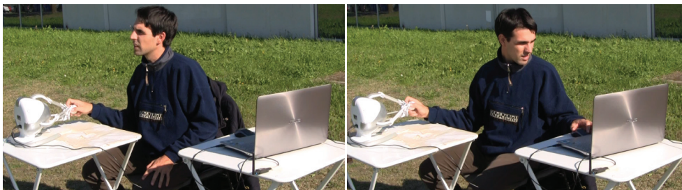
Figure 4.16: An image taken during haptic teleoperation with force feedback enabled (left) and an image taken when force feedback was disabled with pure visual feedback of radioactivity data displayed on the screen of the ground station (right).
