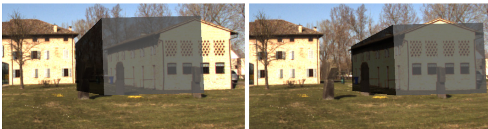
Figure 5.9: Building visualization in augmented reality: result from coarse registration (left) and after manual correction (right).
