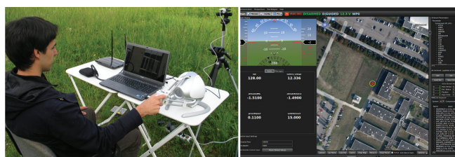
Figure 4.10: Ground station with haptic device (left) and QGroundControl program (right).
