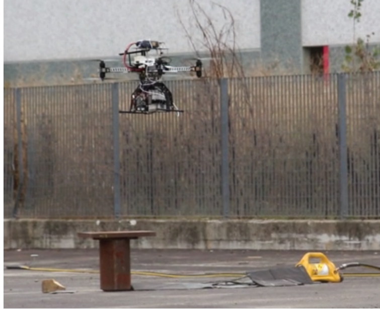
Figure 4.5: UAV equipped with CdZnTe X-ray detector in a flying test in a real environment.
