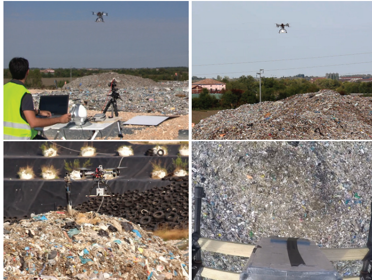
Figure 4.20: Test in a real application context: haptic teleoperation of X-ray detector equipped UAV in a garbage dump.
