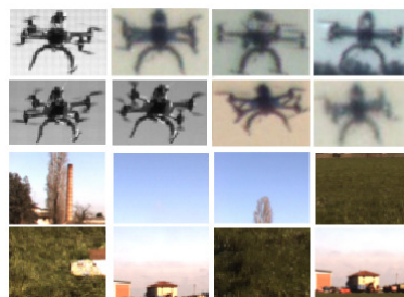
Figure 5.6: Examples of the images used in the training set for vision-based UAV detection.
