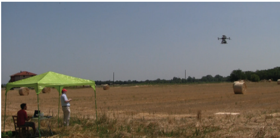
Figure 4.9: Teleoperation experiment in an open grass field. The sensor equipped UAV measures background radiation.
