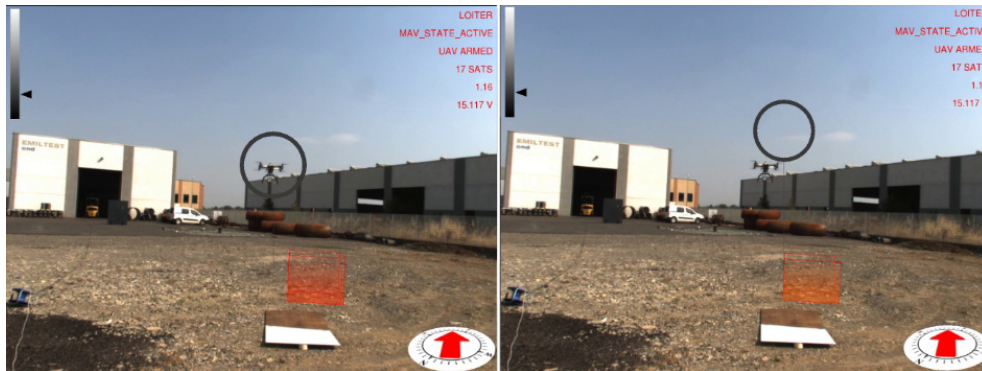
Figure 5.8: Comparison of UAV position estimation methods: vision-based (left), EKF (on-board sensors) (right).
