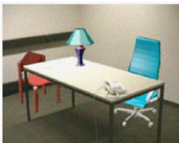
Figure 1.1: Example of AR scene: a real desk and real telephone with virtual chairs and virtual lamp [2].
