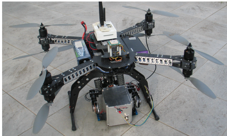
Figure 4.4: UAV equipped with CdZnTe X-ray detector (mounted at the bottom).
