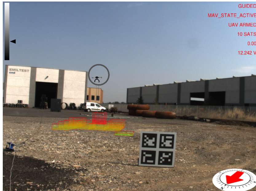
Figure 5.10: Simulated environment developed for the usability tests. The UAV is a 3D model simulated using the ArduCopter SITL simulator.
