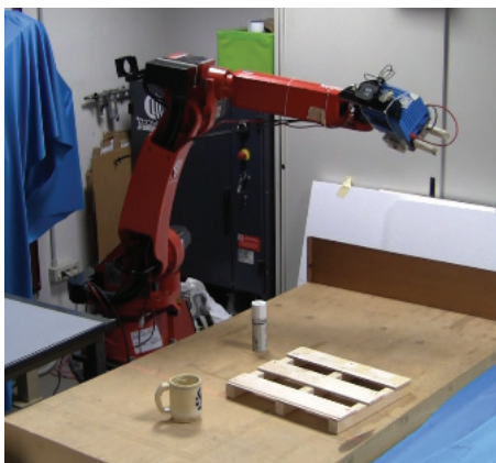
Figure 3.13: Experiment 1: pallet arrangement. Robot laser scan phase.
