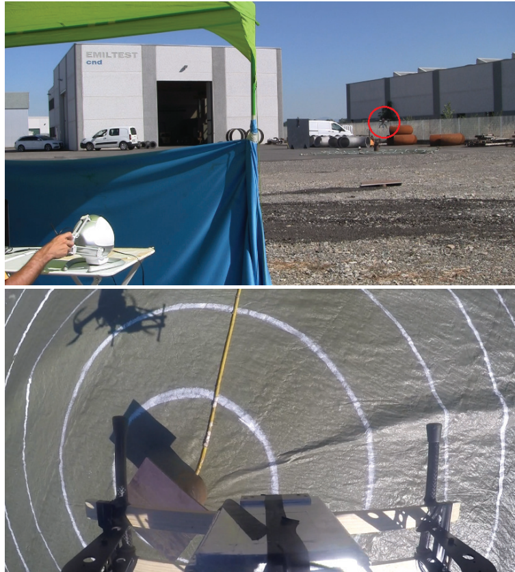
Figure 4.19: Detection of Iridium 192 in real environment using the position-position teleoperation mode. Experimental setup (top), where the UAV is highlighted by the red circle. Image taken from the onboard camera (bottom) when the operator affirmed that the current position of maximum measured radiation was close enough to the real nuclear radiation source (located at the center of the target within the lead container). The cloth in front of the operator prevented him from seeing the location of the nuclear source on the ground. In this set of experiments the gimbal unit was not used to get a clearer view of the ground from the onboard camera. The low speed of the UAV ensured that the X-ray detector remained parallel to the ground during the mission.
