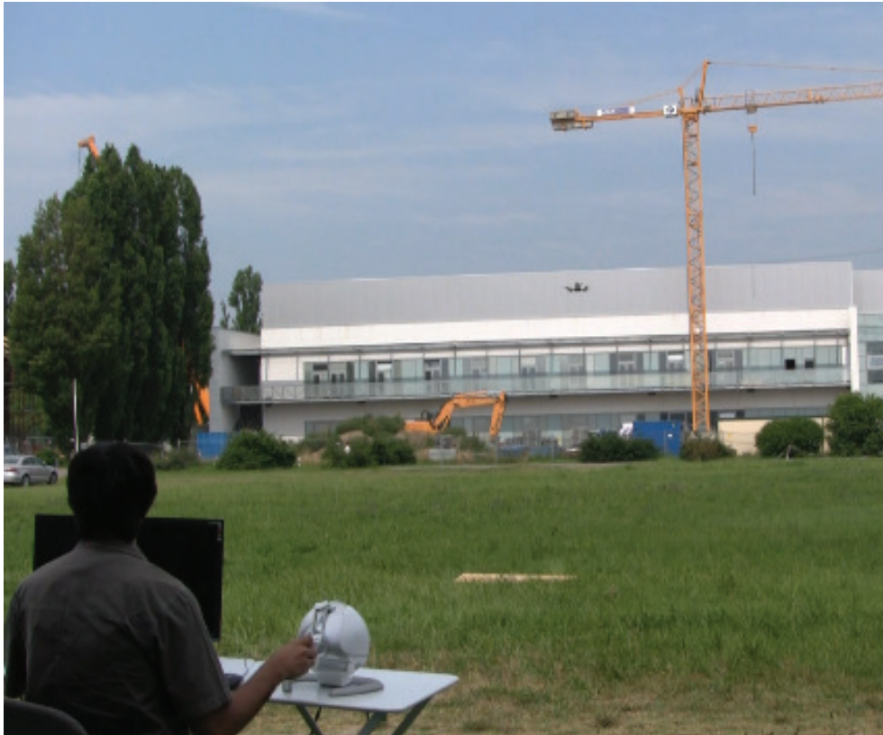
Figure 4.11: A teleoperation experiment using a small UAV with simulated radiation sources and haptic feedback.
