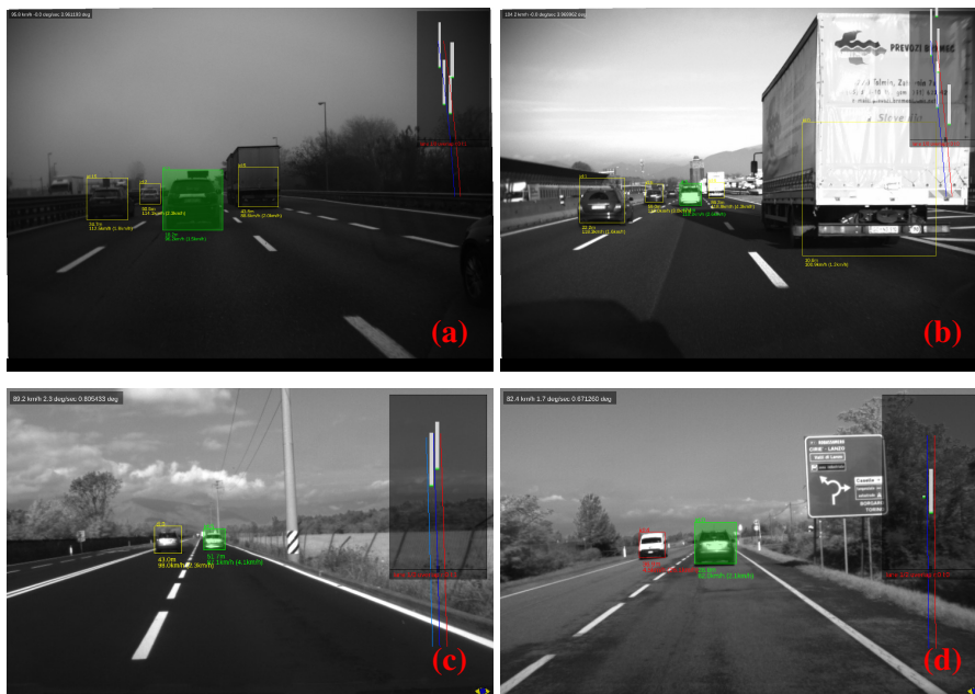
Figure 4.7: In these images is shown the output of the system, each vehicle detected is represented with different bounding boxes: green for vehicles belonging the same lane of host vehicle, yellow for vehicles in the same direction of host vehicle but different lane, red for vehicles in opposite direction. (a) and (b) are referred to TME Motorway Dataset, (c) and (d) are referred to our dataset.
