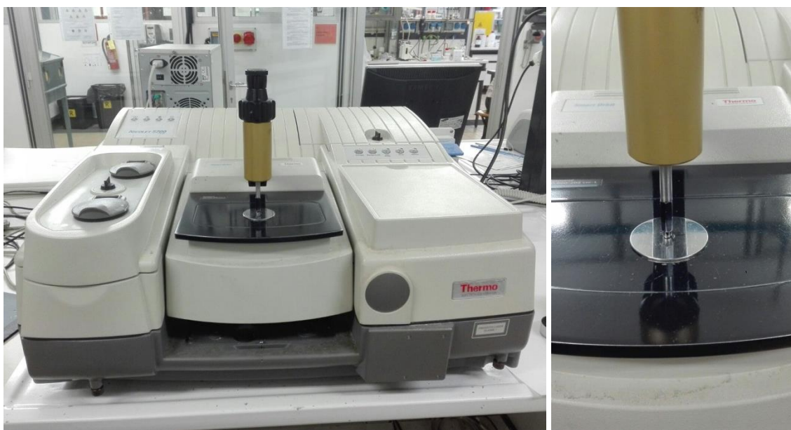
Figura 3.14 - Nicolet FPCFT-IR (ThermoFisher Scientific)
