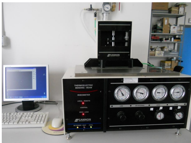
Figura 3.2 - Bending beam rheometer (CANNON Instrument Company)
