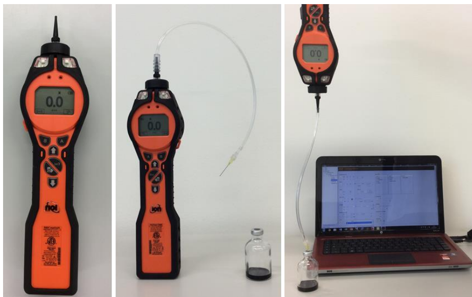
Figura 4.2 - PhoCheck Tiger (ion Science)
