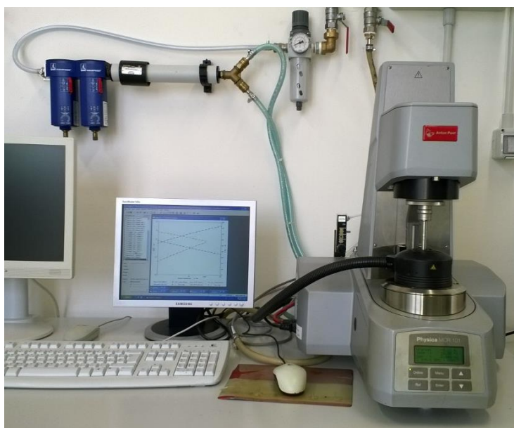
Figura 3.1 - Dynamic shear rheometer (Anton Paar Physica MCR 101)
