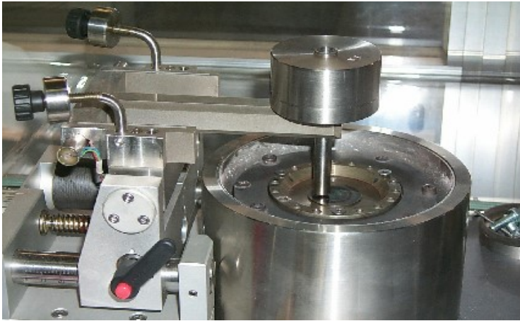
Figure 117. (Left) CSM tribometer available at CNR-IMAMOTER in Turin. (Right) Table with the features of the tribometer.
