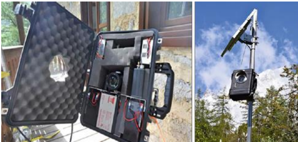
Figure 4.10: Left the watertight IP67 box housing the system. Right one of the system units and the solar panel installed on a pole
