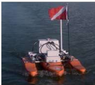
Fig. 1 – The Unmanned Surface Vehicle SWAP (Shallow-Water Prospector), designed and built at ISMAR-CNR in cooperation with Consorzio Proambiente (Tecnopoli dell'Emilia Romagna).
