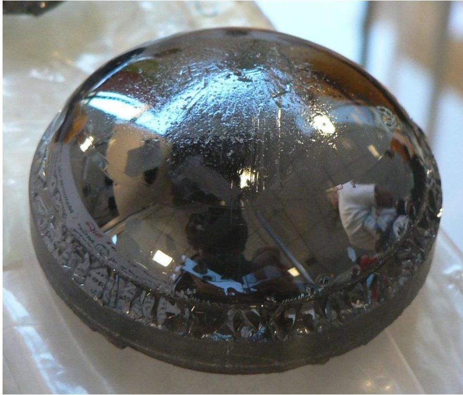
Figure 2.1: Silicon carbide (SiC) monocrystal from the LMGP (Minatec) lab of Grenoble. Author: David Monniaux. Source: Wikipedia (en).
