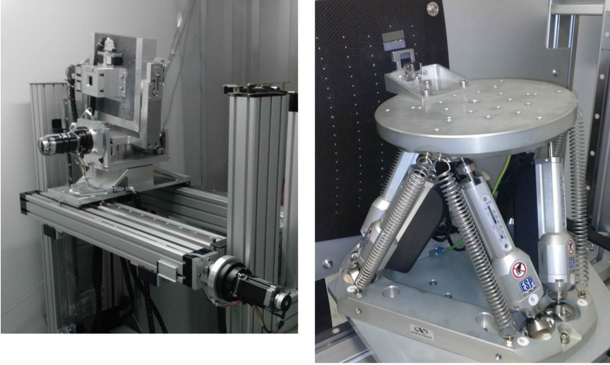
Figure 6.2.4: Left : Collimator and carriage. Right : the hexapod system that is used to tilt and place each crystal in the proper position.
