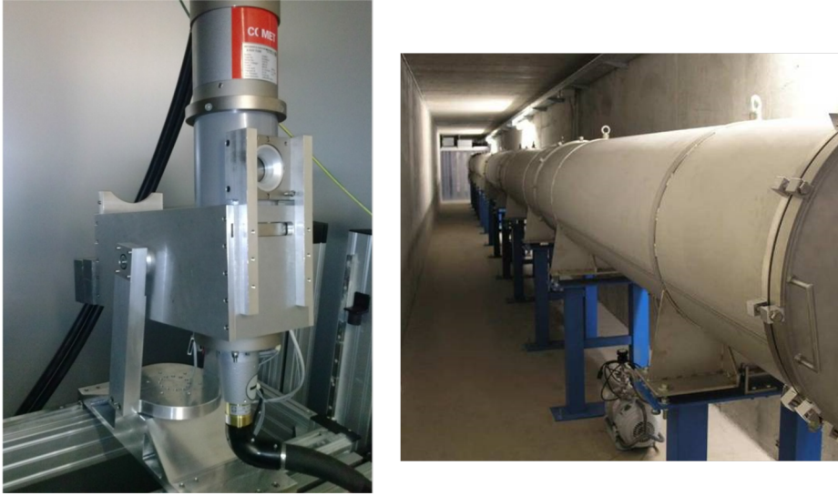
Figure 6.2.3: Left : The X ray source used for assembling and testing the lens petal. Right : The 21 m beam line in which is carried out the vacuum for avoiding absorption and scattering.
