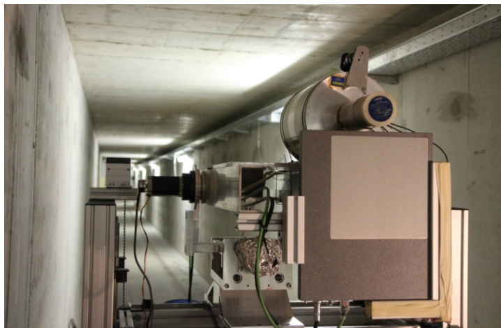
Figure 6.2.6: The two detectors used in the LAUE project: the flat panel detector is positioned below the HPGe detector.
