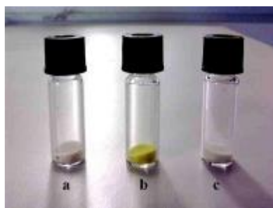
Figure 31 a) as prepared catalyst; b) used catalyst; c) recovered catalyst washed with HCl aq 2 N.
