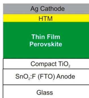
Figure 1.7 Schematic representation of a p - i - n planar heterojunction solar cell using a perovskite thin film both as light absorber and charge transporter. From [35] .
