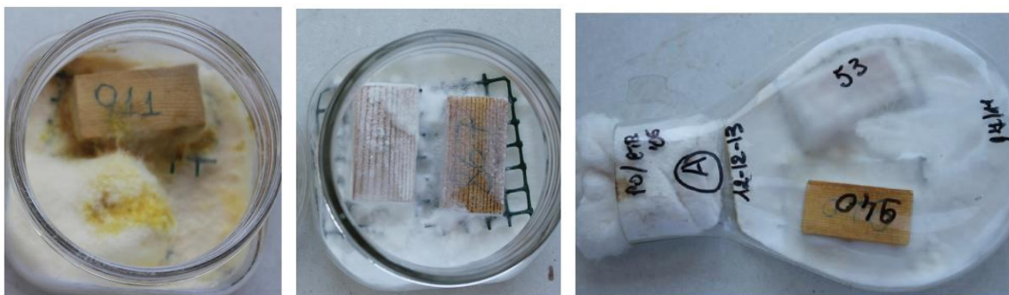
Fig. B.43 – SiPAA - Left, fungus C. puteana , sample 911 (treated) and 40 (control). Center: T. versicolor , samples 867 (treated) and 54 (control). Right: P. placenta , samples 940 (treated) and 53 (control).
