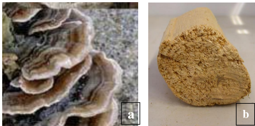
Fig. B.5 – (a) The white rot fungus Trametes versicolor (L.:Fr.) Pilat; (b) White rot decay.
