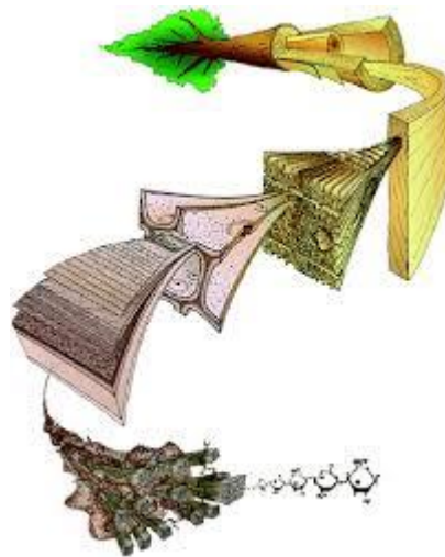
Fig. B.1 - Hierarchical structure of wood ( www.forestplatform.org /Tobias Köhnke).
