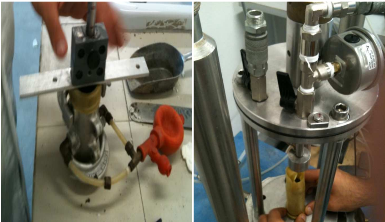
Figure 6.5 The triaxial reconstituted specimen (d = 38 mm, h = 76 mm)
