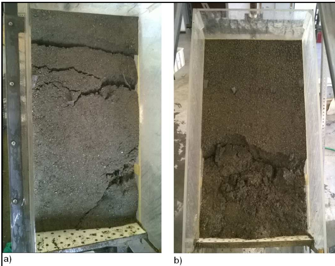
Figure 7.11 Post-failure images of tests with presence of infiltration channels and “Giampilieri scaled hyetograph”. a) test 26, w = 4\% b) test 28 w = 8\%
