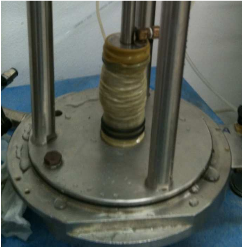
Figure 6.7 The specimen at the end of compression. The specimen assumes the typical “barrel shape” configuration of loose sands.
