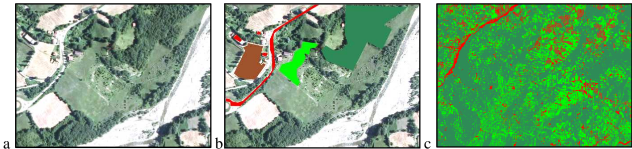
Figure 5.10 Example of image classification: a) a detail of the AGEA flight image, b) examples of training sites of the four classes c) output of the program in which all pixels are classified in one of the four categories.
