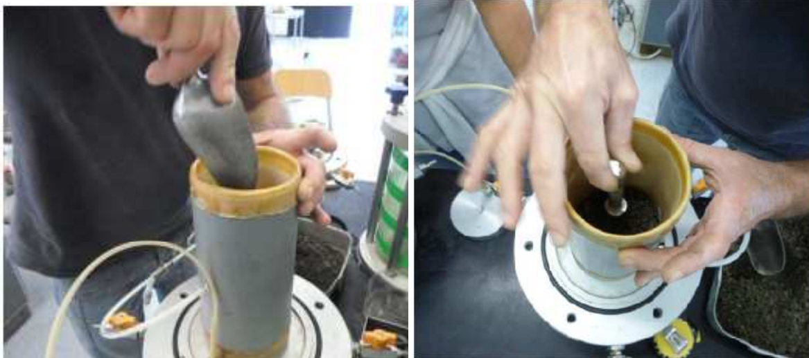
Figure 6.11 The triaxial reconstituted specimen (d = 100 mm, h = 200 mm)
