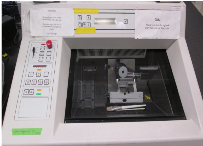
Fig.26 - Leica CM3050S Cryostat for cutting frozen sections.
