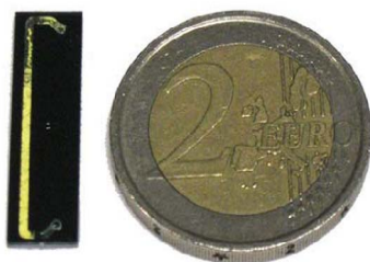
Figure 24. The “trap” filled with crystalline for of the Et-QxBox receptor with 2€ coin for size indication.
