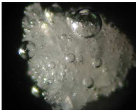
Figure 37. A picture of 24-PF 6 evacuated crystal and then deep in CH 2 Cl 2 . From picture it is possible to show the air bubbles derived from the empty cavities.
