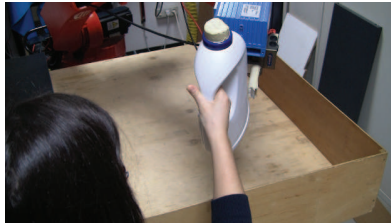
Figure 2.28: Image of a handover experiment from user's point of view. The jug is delivered to the user in a comfortable way by orienting the handle towards the human torso.
