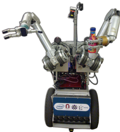
Figure 2.1: HERB, the Home-Exploring Robotic Butler.
