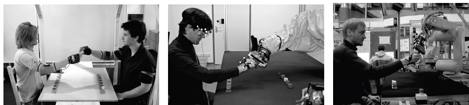
Figure 1.6: Handover experiments (from [47]): left: human-human (Experiments 1, 2, and 3), middle: human-humanoid robot (Experiments 4a and 4b), right side: human-industrial robot (Experiments 5a and 5b).
