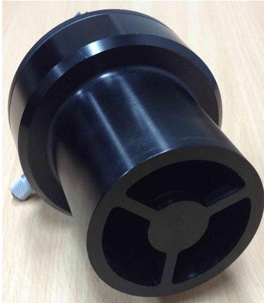
FIGURE 2.27: The finite conjugates catoptric optical head of the scanner
