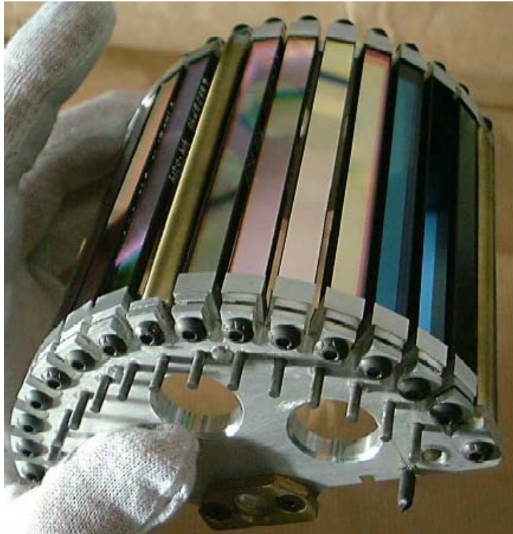
FIGURE 2.11: Cask containing the 13 filters of the CRISATEL instrument
