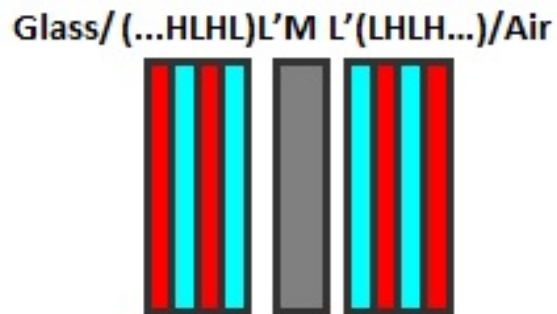
FIGURE 3.10: Schematic architecture of the stack of layers forming the INDUCED-TRANSMISSION LVF
