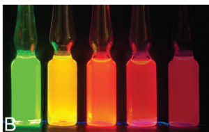
Figure 2.5: Micromolar aqueous suspensions of 525, 565, 585, 605, and 655 quantum dots (left to right) under UV illumination.
