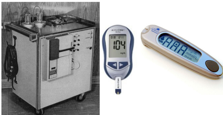
Figure 1: On the left the glucose sensors proposed by Clark and Lyons [3], while on the right two glucose sensors commercially available nowadays.
