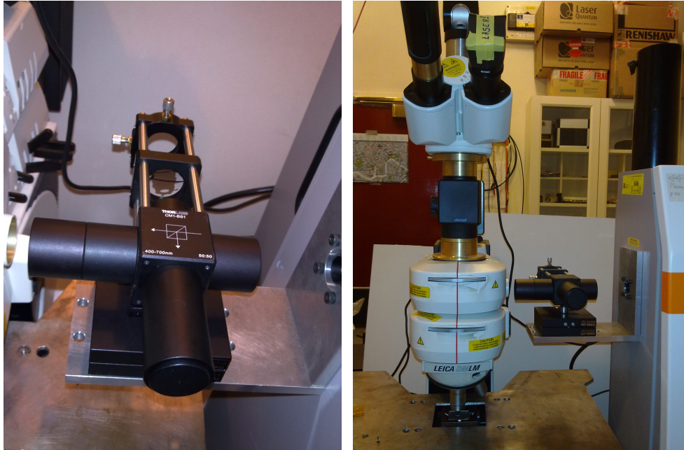
Figure 3.2 – The beamsplitter cased in an aluminum box and mounted on a support to be fixed on the laser path (left). The detector is not shown here. The final arrangement used for thermoreflectance measurements (right): from left, the confocal microscope, the beamsplitter section, and the laser source.
