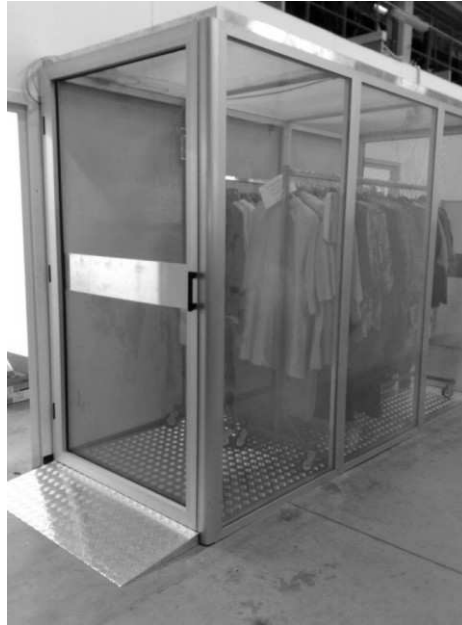
Fig. 18: RFID Cage installed at the DC.
