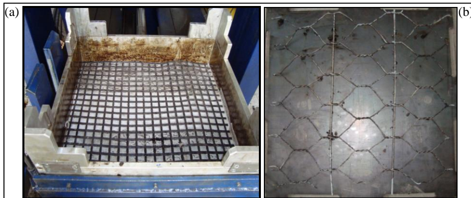
Figure 1.10 Reinforcing systems positioned in the formwork: steel net (a) and glass grid (b).
