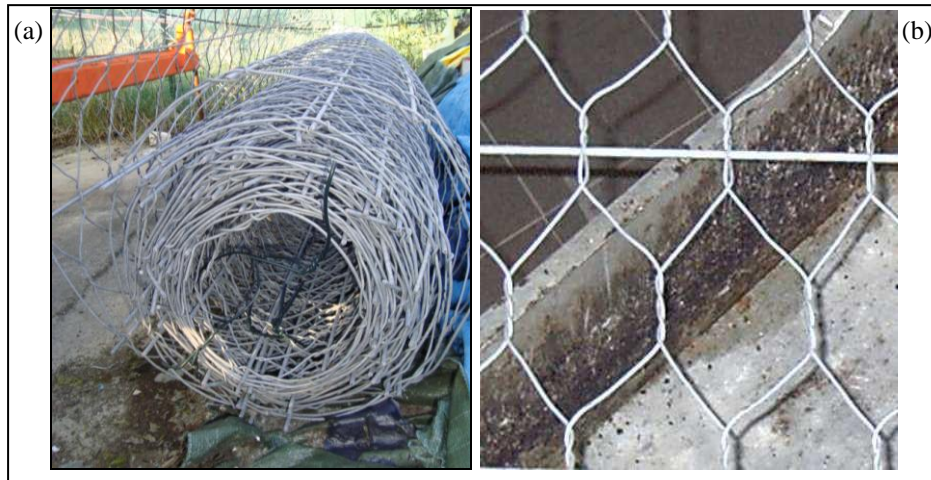
Figure 1.8 Steel net reinforcing system (a) and a detail of the double twisted grid.
