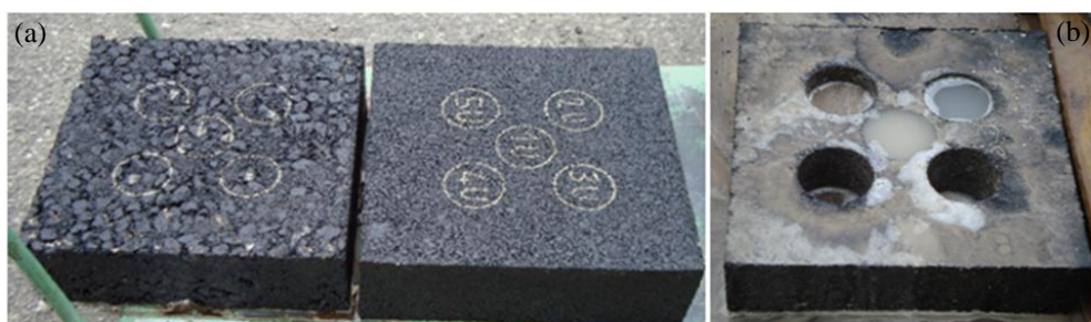
Figure 1.6 Slabs compacted (a) and cored (b) to obtain cylindrical samples.
