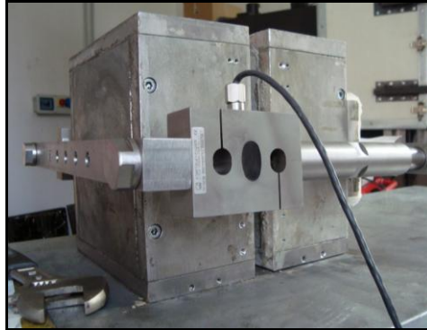
Figure 1.12 “Fixing procedure” for the preparation of the shear test samples.
