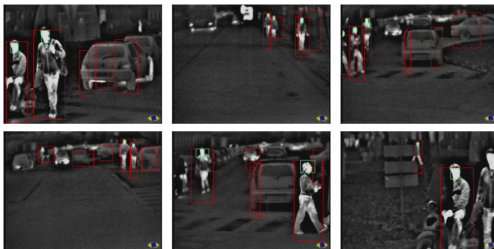
Figura A.37: Results of the head detector validator: green bounding boxes show heads detected inside the original areas of attention in red.
