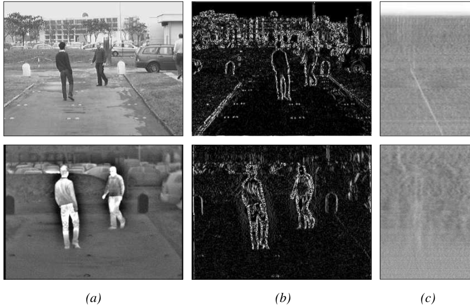
Figura A.2: V-disparity computation in visible and infrared domains: (a) original images, (b) Sobel images, and (c) V-disparity image.
