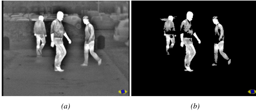
Figura A.3: Preprocessing phase: (a) original input image, (b) focus of attention.
