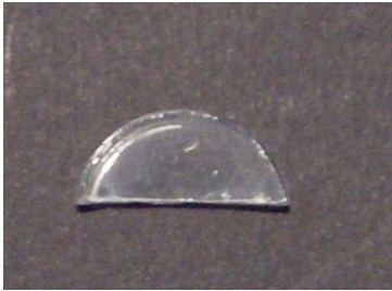
Figure 5.1 Picture of the \text{SiO}_2: \text{Eu}^{3+} 0.001mol% sample: it is characterized by a “foggy” region on the left.
