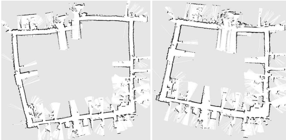
Figure 4.8: Map of the environment of dataset ACES before (left) and after (right) a loop closure is solved with ScanMap .
